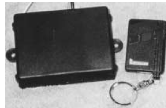
Remote control engine shut-off and receiver.
