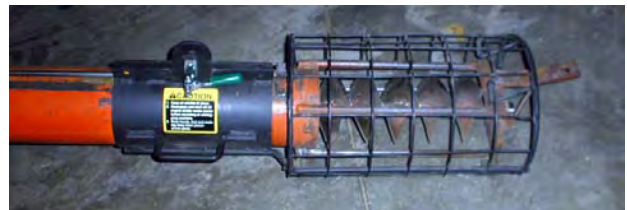
Figure 2. Guard in working position (note warning decal).
