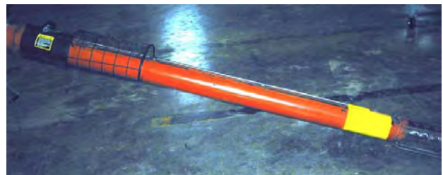
Figure 3. Guard temporarily slid up auger.
