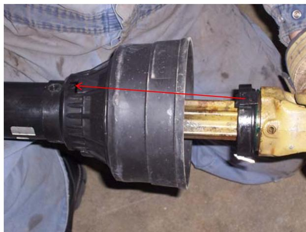
**Figure 3.** Tabs Around the Circumference of the Nylon Bearing Line Up With Holes Around the Bell; Once the Tabs are Inserted in the Holes, the Tube and the Bell Become Integral With the Bearing.
